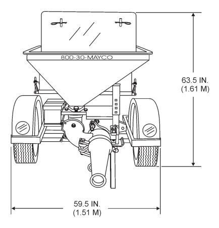
Figure 1. C-30HDNI Concrete Pump Dimensions
